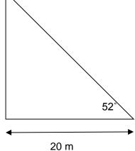
Calculate the height of the mobile phone mast. Round your answer to 1 decimal place. Do not use a scale drawing.
