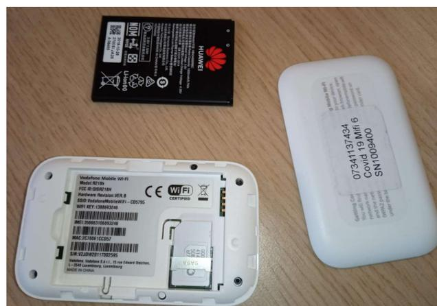
The MiFi hotspot has a Vodafone 4G Sim card, a power supply to charge the device and a battery when working remotely. As long as the phone signal in your location is good, you will get internet access using your MiFi hotspot.
